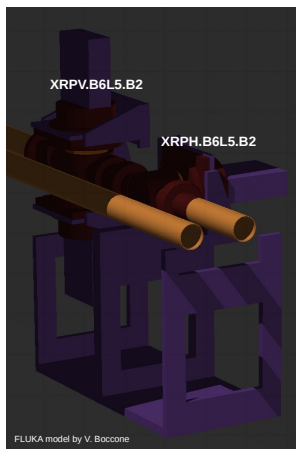
Figure left: FLUKA model of Roman Pot Unit for TOTEM in IR5
