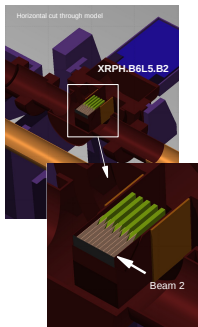
Figure left: FLUKA model of Roman Pot Unit for TOTEM in IR5 Figures right: horizontal cut through XRPH.B6L5 and focus on jaw
