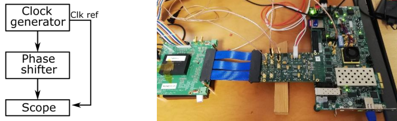
Figure 8. Diagram of test setup, and the picture of the test setup. The linearity and jitter performance were tested along with PLL. The internal PLL provides a 640 MHz, and a 40 MHz clock. The control bits are connected to the I2C module and controlled by the I2C bus. The phase shifter was tested by a high sampling rate electrical oscilloscope.
