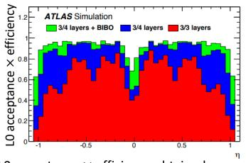
LO acceptance  $\times$  efficiency obtained with respect to offline reconstructed muons
