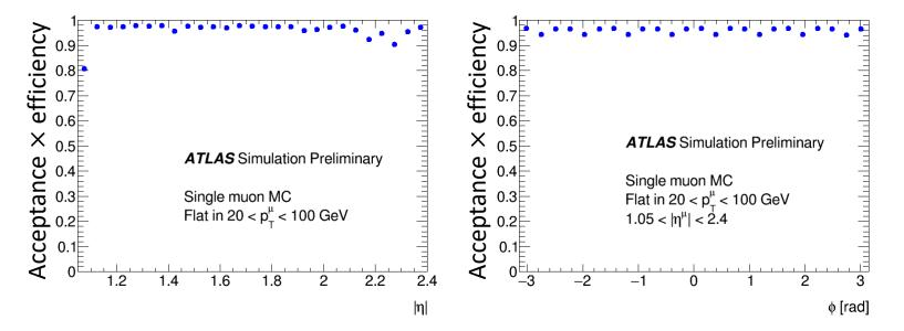
Smaller efficiencies in several bins ( $|\eta| \sim 1.4$  and 2.2, one out of three  $\phi$  bins) due to TGC detector holes for the laser paths of the MDT alignment system
