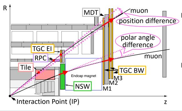
Position difference  $(\eta, \phi)$ : between track segment reconstructed from TGC BW and hits from TGC EI, RPC and Tile
