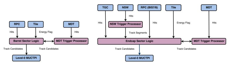
Barrel and endcap SL boards have a common hardware design.
