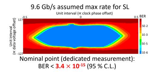
Result of FireFly loopback test with Xilinx IBERT
