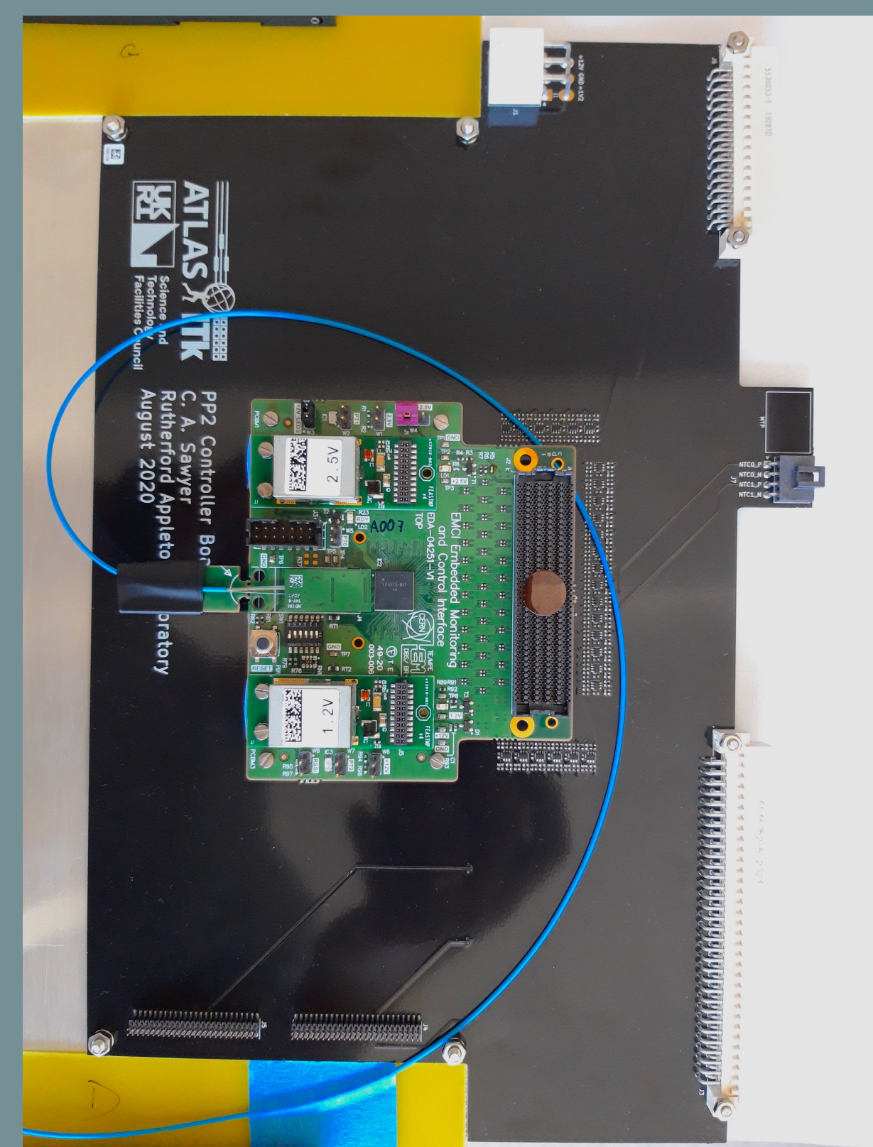
Crate controller system (lpGBT-based).
