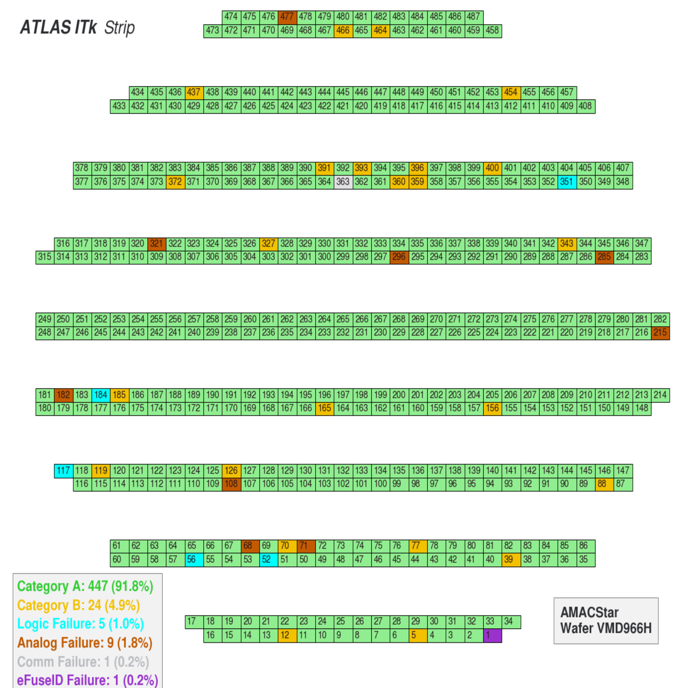
Figure 8: Example wafer map from one of the production priming wafers [ITK-2022-02]
