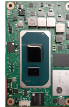
COM Express Mini Module Type10 Intel® 11th Gen Core Processors 8 or 16GB LPDDR4 NVMe SSD, PCIe Gen-4 USB 4
