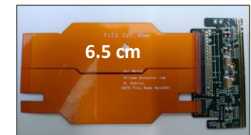
6.5 cm long flex cable tail prototype for the demonstrator attached to a module flex prototype
