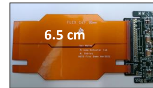
Flex cable tail prototypes for the demonstrator 13 lengths : 73.2-28.5 cm long (longest and shortest length)
