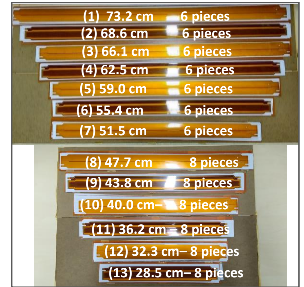
Flex cable tail prototypes for the demonstrator 13 lengths : 73.2-28.5 cm long (longest and shortest length)
