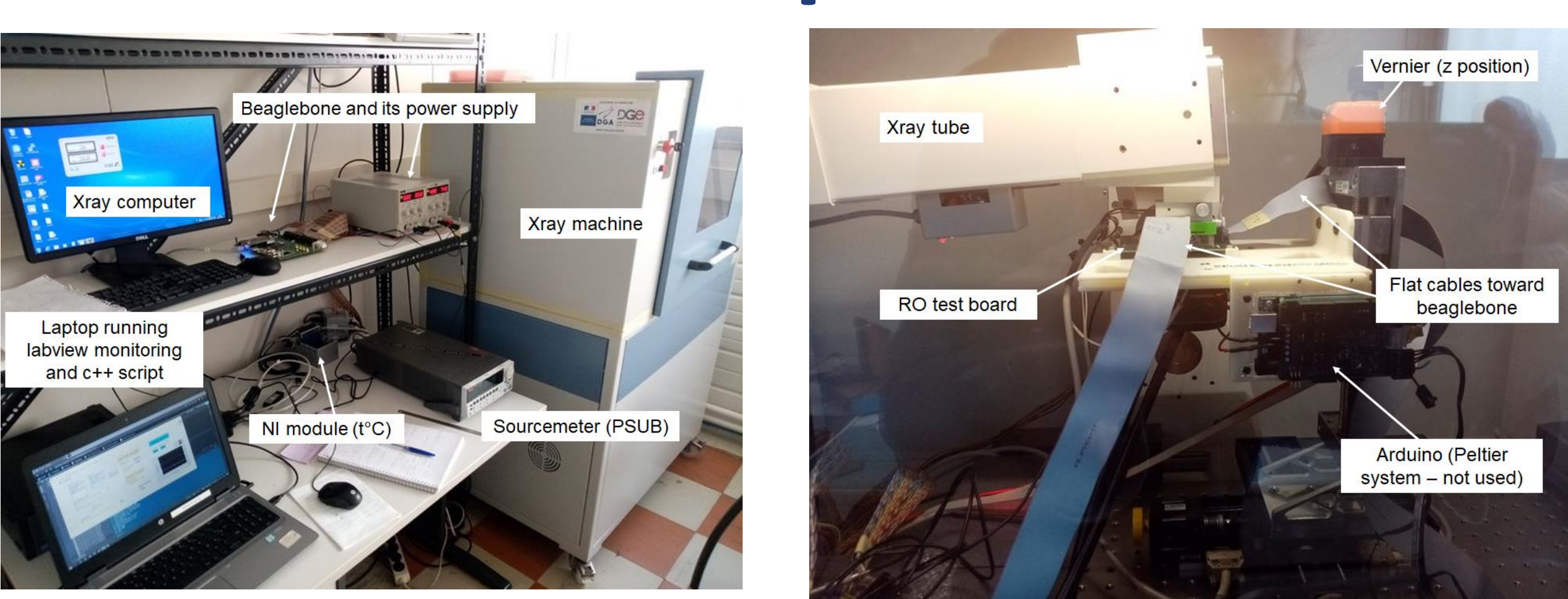
Fig7. Left: global view of the irradiation setup. Right: installation inside of the X-ray machine.
