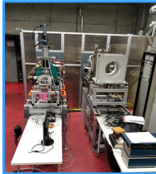
Two benches connected to HV cage
