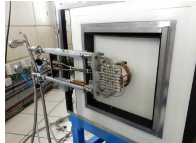
Beryllium target + cooling inside ½ moderator + shielding
