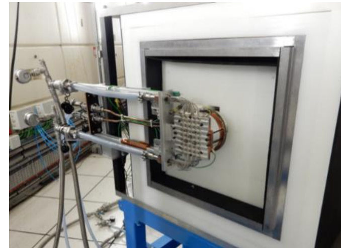
Beryllium target + cooling inside ½ moderator + shielding
