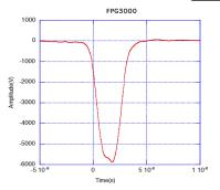
Pulse width(FWHM) = 2ns Pulse height = 5.8kV Rise time = ~1.5ns(5%~95%) Time jitter = ~29ps Amplitude Jitter = 0.72% (limited by the scope resolution)
