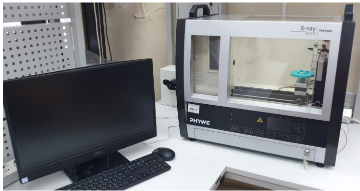
Setup for measuring spectrum of X-rays using Bragg's diffraction
