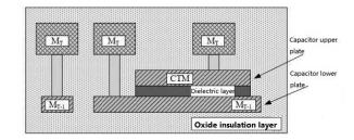
MIM use different layers of metal and interposed dielectric to form a capacitor. Similar to plate capacitor, good stability but require additional masks
