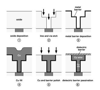
Dual Damascene\* process. An additional metal barrier (W) is deposited first to avoid Cu contamination of Si. Cu deposited by electroplating. CMP is needed as Cu does not plasma etch.
