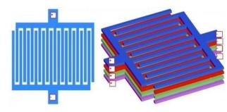
*MOM use interdigitated capacitors formed by metal connections, placed in close proximity – preferred choice for advanced CMOS, also no additional mask required*
