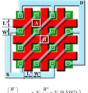
$$\left(\frac{W}{L}\right)_{\text{WAFFLE}} = N_{\text{A}} \frac{W'}{L'} + N_{\text{B}} \left(0.55871\right)$$
