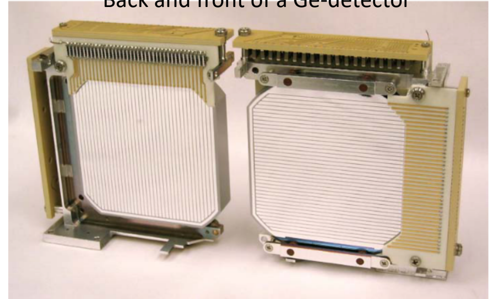
Back and front of a Ge-detector
