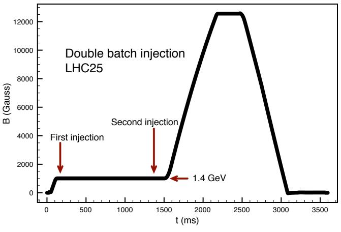
Depending on the bunch spacing or the intensity per bunch, the LHC beams are produced taking one or two extractions from the PSB.
