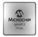
FPGA (Field Programmable Gate Array)
