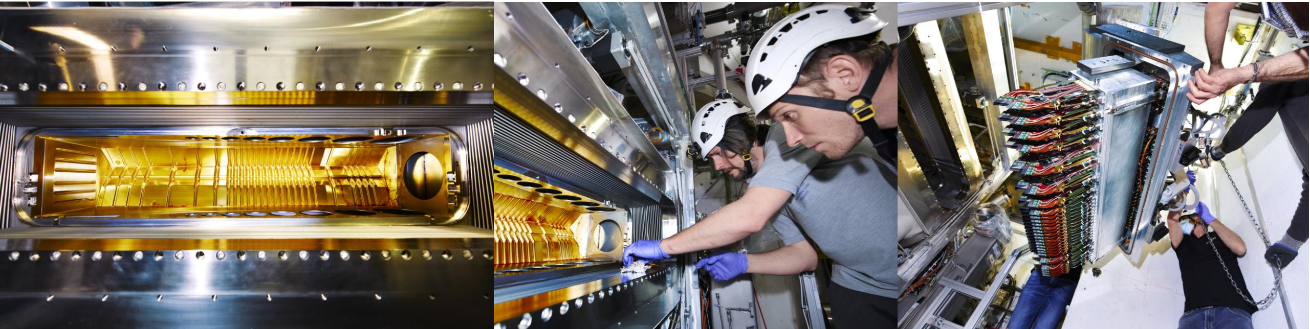
Installation of the VELO A-side
