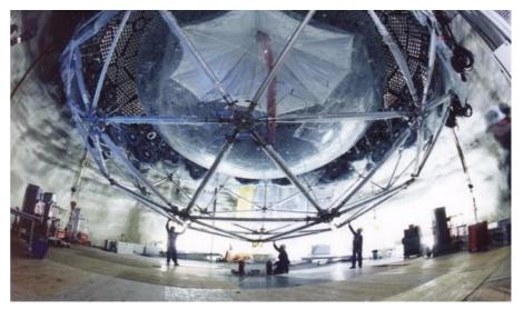
1000 tonnes of  $D_2^0$ 6500 tons of  $H_2^0$ Viewed by 10,000 PMTS In a salt mine 2km underground in Sudbury, Canada
