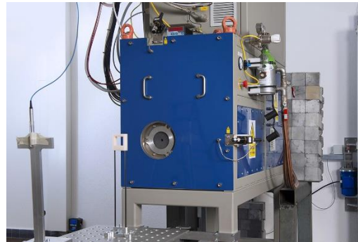
eRT6 Oriatron PBM/Alcen Electron beam, 5.5 MeV energy Pulsed beam
