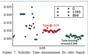
Figure 7: Schottky Tune measurement for pilot bunch (blue), nominal bunch with 1 collision (red) and nominal bunch with 2 collisions (green).
