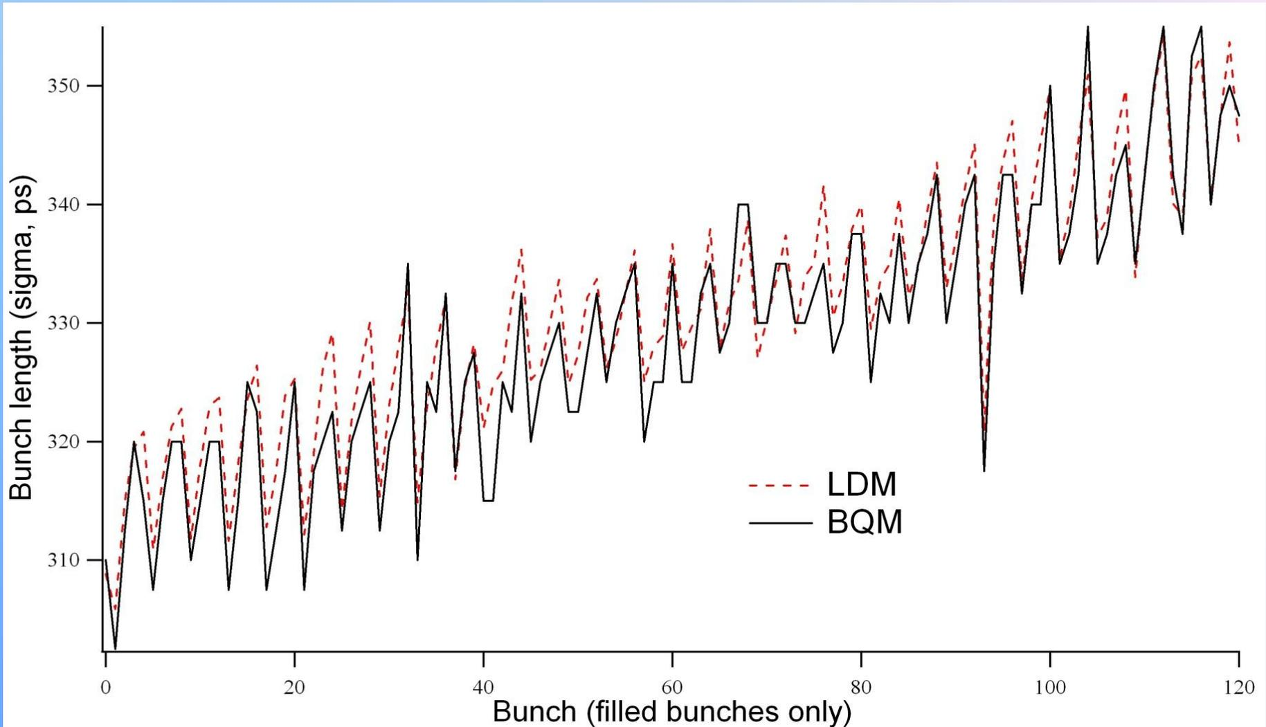
LDM bunch length: Gaussian fit  $\oplus$  90ps LDM time resolution
