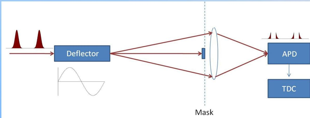
Electro-optic deflector maps longitudinal profile onto transverse plane
