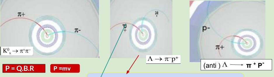
P = momentum Q = electric charge B = magnetic field R = radius of curvature The red tracks indicated positive charge and the green tracks indicate negative charge.
