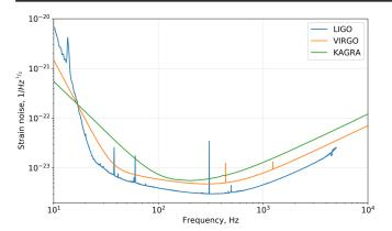
FIG. 1. Projected LIGO, Virgo and KAGRA strain noise (i.e., amplitude spectral density),  $\sqrt{S_n}$  as a function of frequency for the fourth observing run O4. The data used to generate the noise curves above are retrieved from [48].
