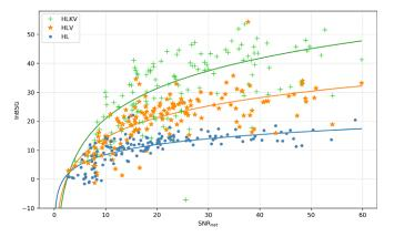
FIG. 7. Log signal-to-glitch Bayes factor  $\ln \mathcal{B}_{S,\mathcal{G}}$  of sine-Gaussian wavelet recoveries versus network signal-to-noise ratio SNR<sub>net</sub>. The solid lines with colors corresponding to the data symbols are analytic predictions of  $\ln \mathcal{B}_{S,\mathcal{G}}$  given by Eq. (C2).
