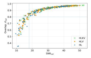
FIG. 3. Median overlap between the injected and recovered waveform  $\mathcal{O}_{net}$  of the HL (blue dot) and HLV (orange star) network, as a function of SNR<sub>net</sub>. The horizontal blue line indicates  $\mathcal{O}_{net} = 0.8$  and the vertical blue line indicates SNR<sub>net</sub> > 15.
