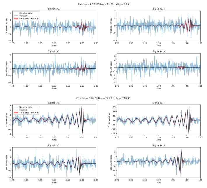
FIG. 4. The top panel shows, for an injection with  $SNR_{net} = 11.61$  and  $\mathcal{O} = 0.52$ , the injected waveform (black line), the detector data (blue line) and the 90% credible interval of the recovered waveform (red line) for each detector in the HLKV network. Similarly in the bottom panel but for an injection with  $SNR_{net} = 52.72$  and  $\mathcal{O} = 0.98$ .
