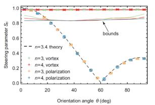
**Quantum** steering versus the orientation angle. Dots are the experimental data, and the lines with corresponding colours steering bounds represent taking into account the number of measurement settings, *n*, and detection efficiency.
