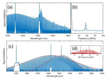
**Experimental realization of soliton linear-waves and multiplexed solitons.** (a) Spectral extension of the soliton comb. (b) RF beat note measuring the relative detuning between the pump and second lasers from resonance via scattering between the soliton and linear wave. (c) Two cavity soliton spectra. (d) RF beat comb with 112 MHz comb line spacing.
