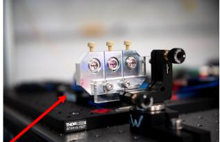
Fibre collimator/partial reflectors
