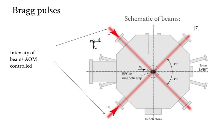
[7] R. I. Khakimov 2016, *Source of correlated atom pairs*, Figure 5.2: Schematic of the Bragg/Raman beams entering the vacuum chamber.
