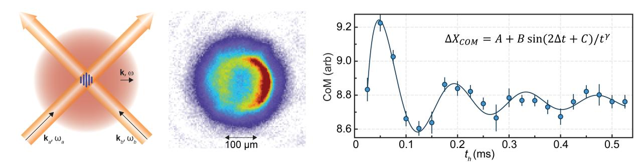
• The **frequency**, **amplitude** and **damping** rate are determined by fitting a **damped sinusoid**.
