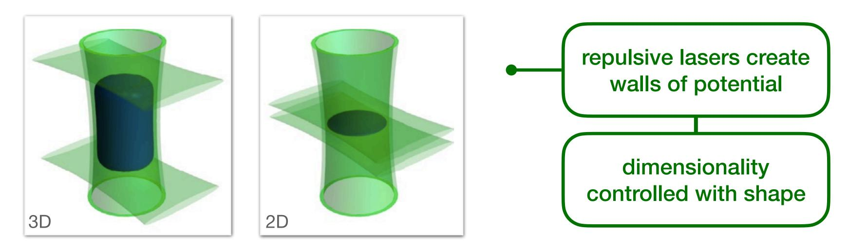
shaped light modulators (SLM) and digital micro mirror devices (DMDs) create optical potentials
