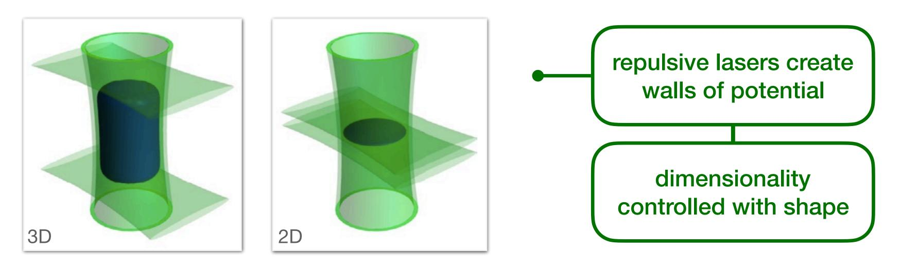
shaped light modulators (SLM) and digital micro mirror devices (DMDs) create optical potentials
