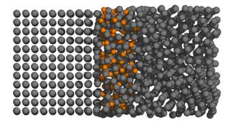
Figure 1: An atomistic Al/AlO<sub>x</sub>/Al Josephson junction constructed using molecular dynamics.
