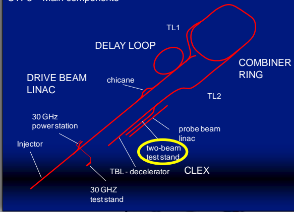
CTF3 – Main components
