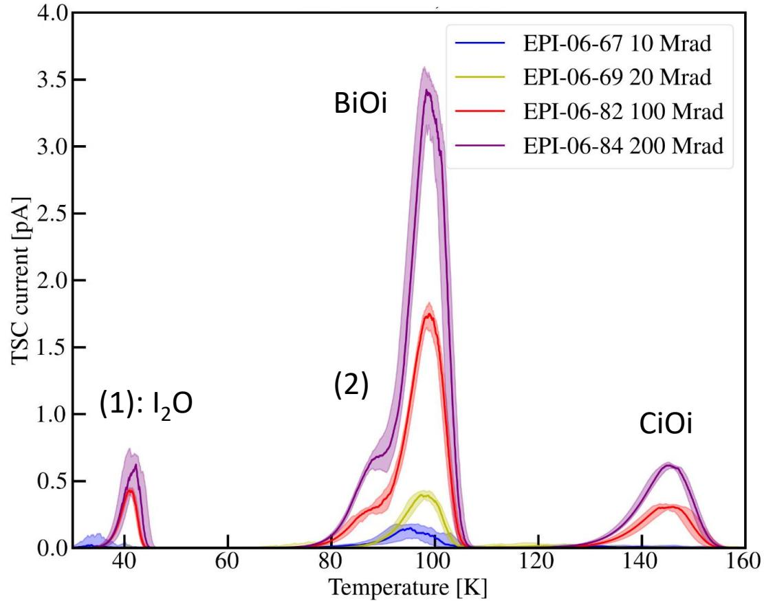
measured TSC spectra (VR=-100V, Vfill=+20V, Tfill >40K):
