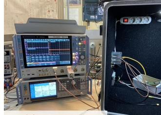
Rohde & Schwarz RTP164 16GHz Oscilloscope and SMA100A 50GHz signal generator
