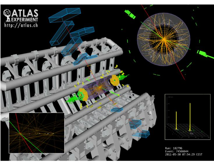
Strategy for this channel (there are several) - we look for events with **two Z bosons** that have decayed to **four leptons**, e.g. two electrons and two muons in the event on the right If the **two Z bosons** were produced by the **decay of a Higgs boson**, when we reconstruct the invariant mass of the system we should see a **peak** at the **Higgs boson mass**
