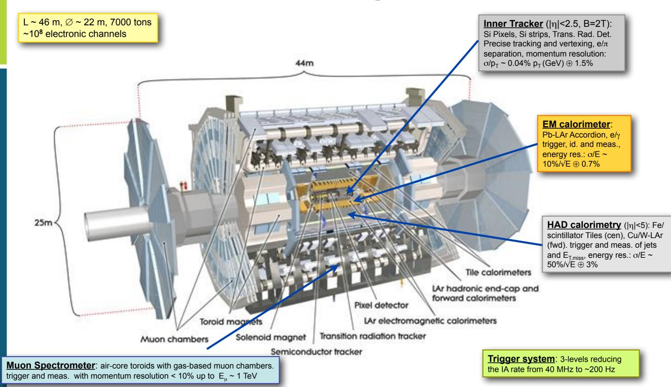
Millions of detector readout channels read out to reconstruct one "event"
