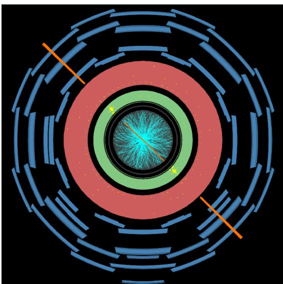
Event displays are great ways for us to visualise what happened in a particle collision. In this **ATLAS** event display (*right*) of a real proton collision, we are looking down the beam pipe, so the plane of the display is transverse to the proton beam direction. **Question**: Can you quantify the momentum in this plane before the proton collision
