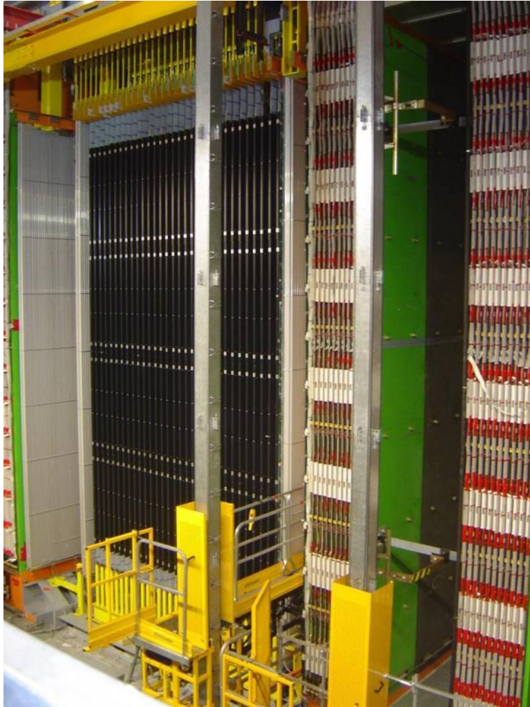
Scintillator planes 5900 \text{ m}^2 8064 7m long drift tubes
