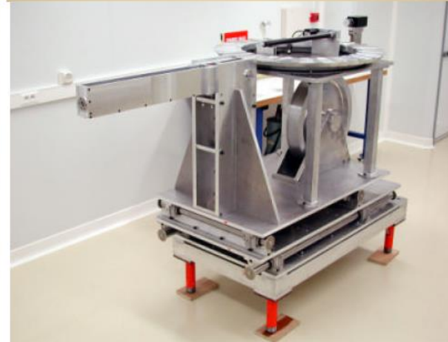
"Carousel" brick dispensing and storage system
