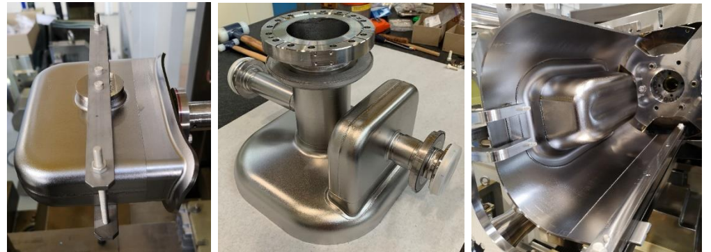
Welding of CRAB cavities at CERN
