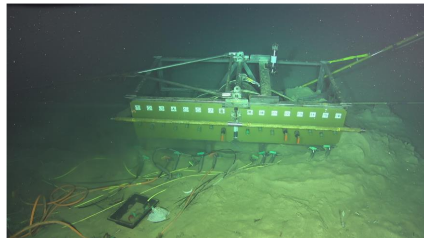
Junction Box 2022, after 20 y in seawater
