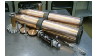
12 GHz klystron and pulse compressor for CERN high-power test stand
