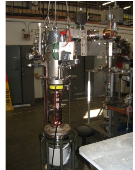
12 GHz klystron and pulse compressor for CERN high-power test stand
