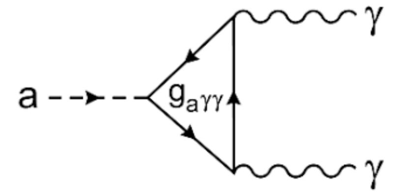
$$\Gamma_a = \frac{m_a^3 g_{a\gamma\gamma}^2}{64\pi}$$
