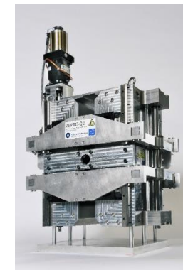
UKRI's ZEPTO tunable PM quadrupole
