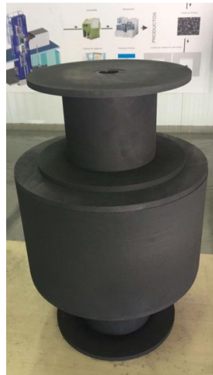
Stress relieving thermal treatment 0 MPa, >2400 °C
