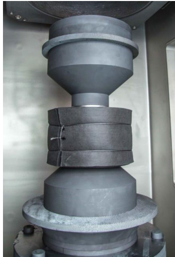
Spark Plasma Sintering (SPS) >25 MPa, >2600 °C
