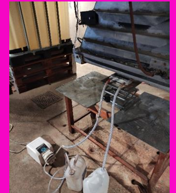
An installation for flow irradiation of sewage sludges under ILU-6 accelerator
