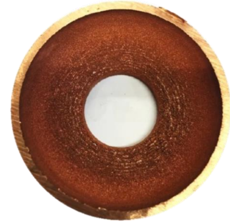
Half cavity printed without any kind of supporting structure
