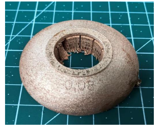
Gap between the supporting structure and the cavity
