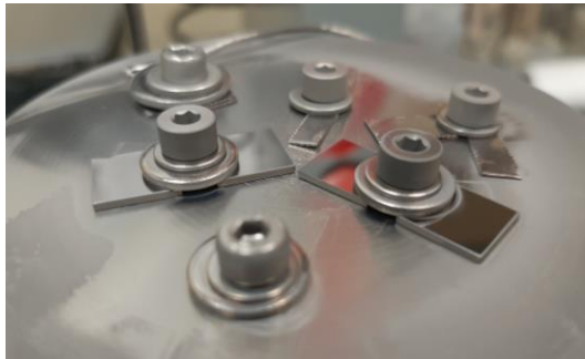
Nb 3 Sn coatings on sapphire, copper and quartz
