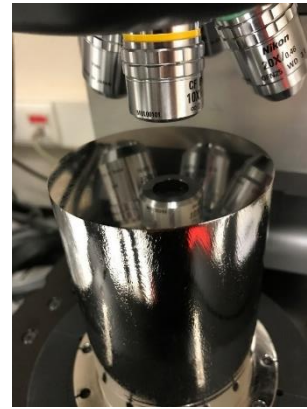
After EP 150 \mu\text{m} + annealed at 900°C under vacuum + EP 20 \mu\text{m} at CEA
