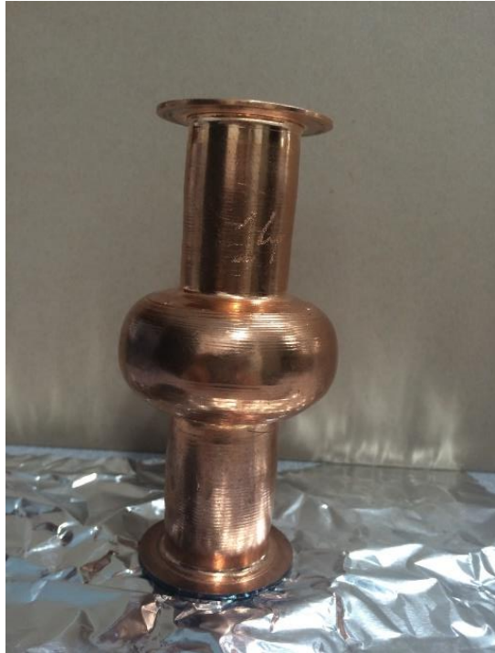
INFN seamless standard elliptical copper cavity
