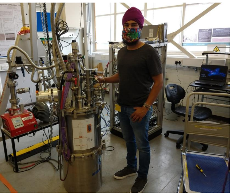
EXP800: RRR, Magnetic field penetration + 2 other experiments (in-He-gas)
