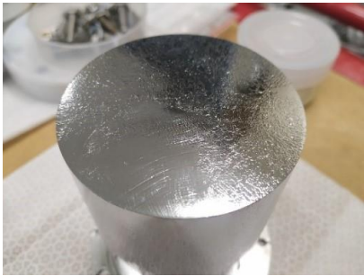
QPR sample milled from ASTM0 large grain material Poor RF performance, In contaminations
