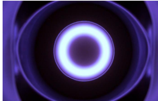
Nb 3 Sn 4" planar magnetron source @LNL
