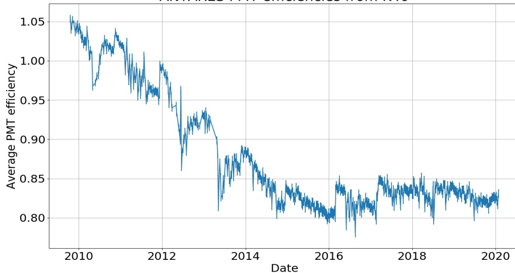
ANTARES PMT efficiencies from K40
