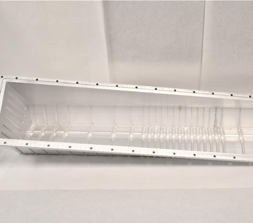
Thinning to 150 \mu\text{m} of the VELO LHCb RF box window
