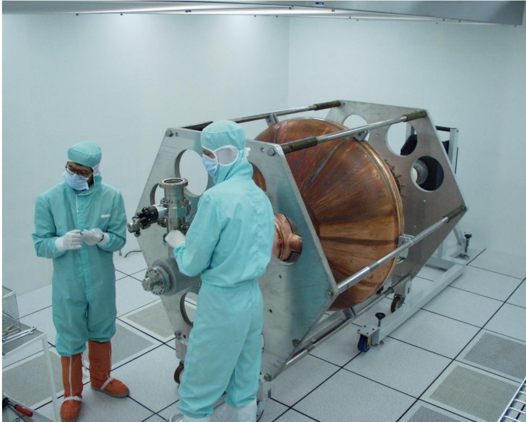
ISO5 clean room for assembly
