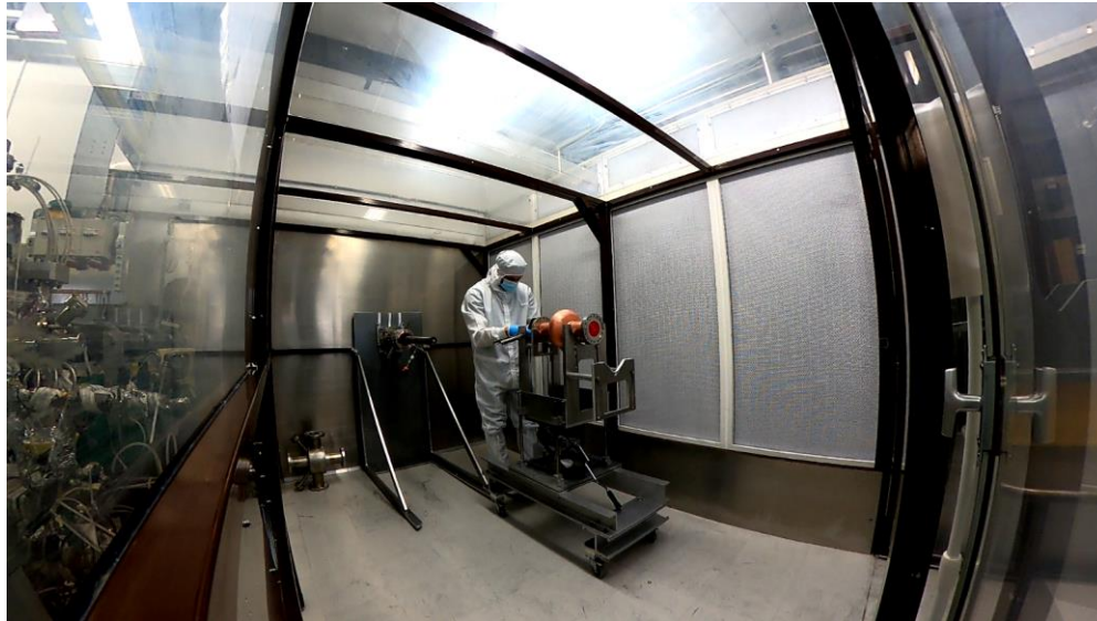
ISO5 clean room for assembly
